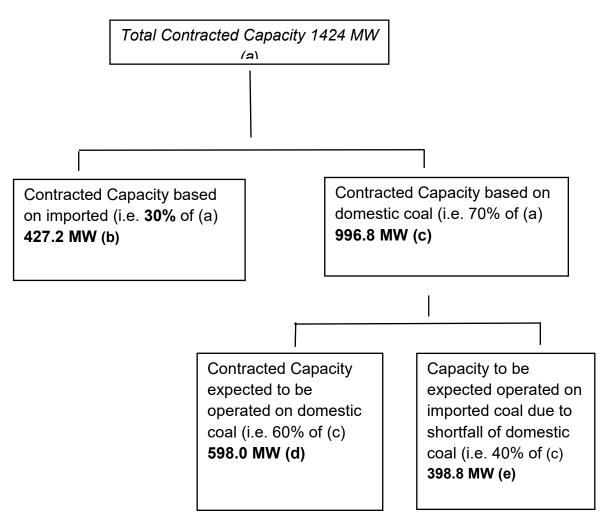
The expected capacity to be operated based on imported and domestic coal:
